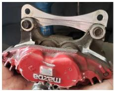
Step 8. Bolt relocation bracket/caliper to hub as shown using provided cap screws and lock washers. Tighten to factory torque specifications. (you may have to run a tap through the threads of the spindle to clean them out as the OEM hardware doesn't run totally through and they often rust there)
