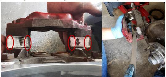
Step 5. Grind/file mounting ears of the brake caliper at a 45\* angle as shown until the clear the hub mounting ears when bolted to the bracket.
