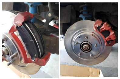
Step 8. Bend brake dust shield back toward original position, making sure that it doesn't contact the rotor.
