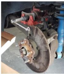
Step 3. Grind down ears of spindle as shown until the FD rotor sits on the spindle flat & freely, being careful to avoid hitting your wheel studs.
