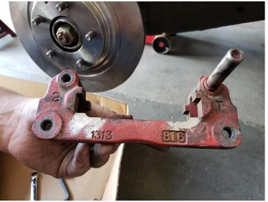
Step 5. Bolt caliper relocation bracket to caliper bracket as shown using provided socket head cap screws and lock washers. Tighten to factory torque specifications. \*
