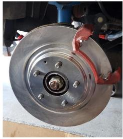
Step 7. Set brake pads in caliper bracket, slide caliper onto caliper bracket and bolt caliper to caliper bracket to factory torque spec. \*
