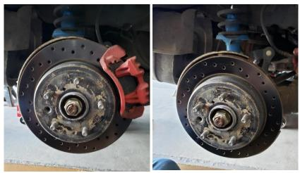
Step 2. Compress the Caliper piston.
