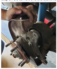
Step 6. Set the FD rotor on the hub and bolt the caliper relocation bracket to spindle at factory caliper bracket location as shown using your OEM hardware. Tighten to factory torque specifications.\*
